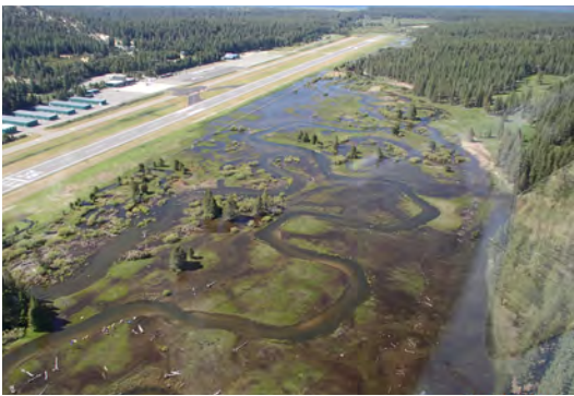
Beginning in 2013, the USDA Forest Service constructed a new channel and recontoured the floodplain to allow spring flows of the Upper Truckee River to spill over its banks and saturate the meadow once again. / Tahoe Regional Planning Agency
