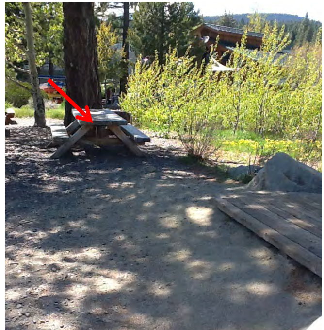
Picnic tables are provided but none are located on an accessible route.
