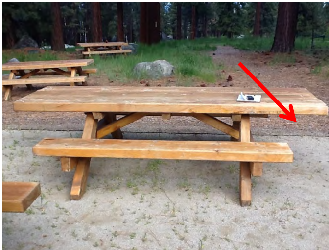
An accessible picnic table must provide a 30"x48" wheelchair space, provide for the allowed knee space within those limits and be located on an accessible route.
