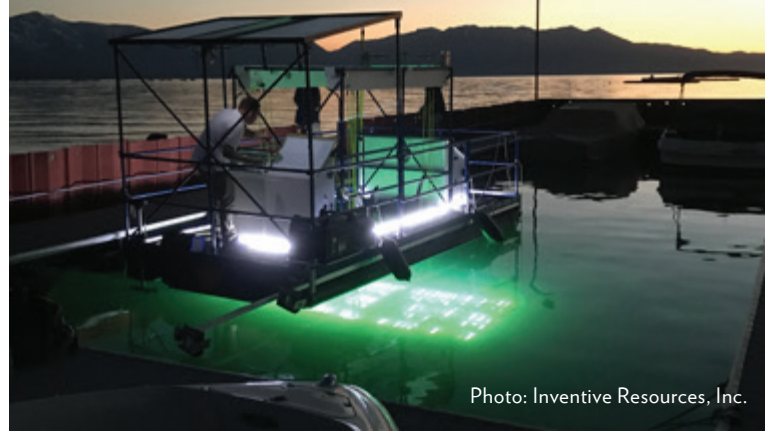
Ultra-violet lights attached to the bottom of this boat are used to kill invasive plants at Lakeside Marina in South Lake Tahoe.
